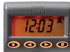
\* If an outside sensor is not fitted the control unit will not indicate battery voltage and outside temperature, but alternate between 24 hour clock - drive away time I - drive away time II at each press on .
